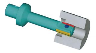
High speed machining of precision bores in volume manufacturing ensures repeatability of bore sizes even after tool changes.
