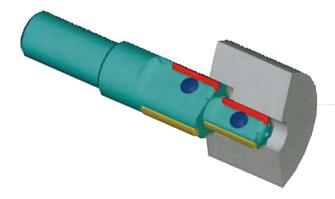
Multi - Diameter reamers to ensure concentricity between bores.
